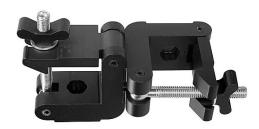
Joins two 2" Square Tubings together. Converts to rigid 90 by changing bolt location. 606 I-T6 Aluminum Alloy. SWL 1200 lbs.
