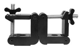
Joins two 2" Square Tubings together. Converts to rigid 90 by changing bolt location. 606 I-T6 Aluminum Alloy.
