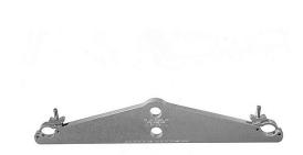
I"  $\times$  6"  $\times$  31-3/8" 606 IT-6 Aluminum CNC machined with pockets to support one piece of 30" truss. Truss is secured by two aluminum pivoting links, half inch swivel bolts, and our solid wing nuts. Has two rigging holes for shackles, motor, or chain hook. The Mega-Truss Pick will suspend one ton of truss, and an additional one ton load suspended under the truss.
