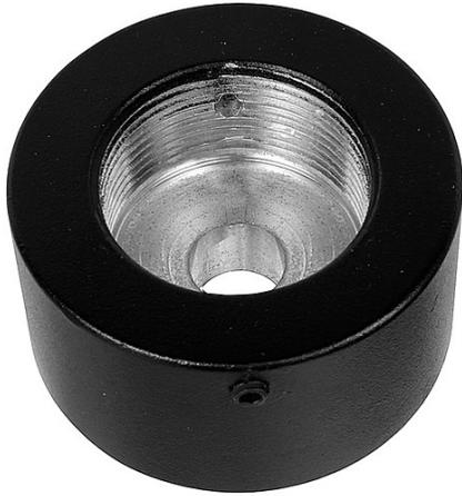
The 5/8" Bolted Truss to Pipe Adapter easily allows joining a pipe to the end of a 5/8" bolted truss. Simply bolt the adapter to the truss with a 5/8" bolt and thread on a 1-1/2" pipe for special requirements. Locking set screw for pipe threads for extra safety.
