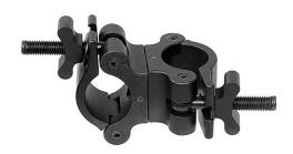
The Mega-Coupler will fasten from 1-1/4" pipe (1.660" OD) to 2.050" OD truss tube. The Mega-Coupler has the wide wing nuts for fastening the clamp to the pipe or tube. Safe Vertical Working Load 1100 Pounds, (500 KG).
