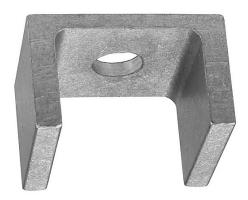
The bar joist washer hooks over the top of bar joists legs up to 1-7/16" wide. The U-shape of the bar joist washer prevents it from slipping off.
