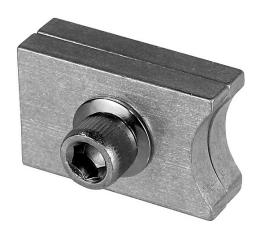
M140 Track Stop for M140 Track. Two CNC machined  $1/4^{\prime\prime}$  ×  $1^{\prime\prime}$  aluminum flat bars with contours that match the curviture of the M140 Curtain Carrier, so as not to "ding" the carrier wheel. The rear bar is threaded for a 5/16" socket head screw to fasten the track stop to the track without needing a nut. The M140 Track Punch will quickly and efficiently add a hole to mount the M140 Track Stop.
