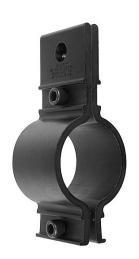
The two-piece, Mega Batten Clamp is great way to hang I-I/2" pipe. The tight compression fit keeps pipe from rotating within the clamp. The Mega Batten Clamp wraps around the pipe batten on both sides and fastens with two 5/16"-18 TPI Socket Cap Screws using a I/4" hex driver. Secure to structural supports through nominal I/2" hole at top of clamp with up to a 7/16" shackle pin, quick link, or turnbuckle jaw. CNC Machined 3/16" thick x 2" wide 6061T-6 Aluminum.
