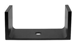
The Mega-Cable Carrier gives you a channel to drop your cables into above the batten or grid. The Mega Cable Carrier has a I/2" mounting hole and is bolted to a clamp. The assembly is then fastened above a pipe batten or grid to run cables. The cables are then located over the pipe, giving you clearance to hang your lights without having to fight the cables, or to worry about messy tie lines.
