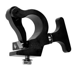
The new standard truss clamp for hanging intelligent lighting fixtures. Allows one man to hang intelligent fixtures. Simply flip the link up, place the clamp over the pipe and the Mega-Claw holds the weight of the fixture while you secure it with the solid 3/4" thick handle. The Mega-Claw will fit onto (I-I/2" Pipe) I.9" OD to 2" OD.
