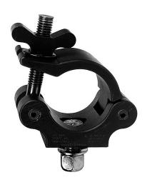
The Mega-Coupler has solid wing nut tabs that are stronger than regular steel wing nuts. The grade 8 Hex Head Cap Screw locks securely into the hex milled pocket so that the nylock nut can be tightened while the damp is installed
