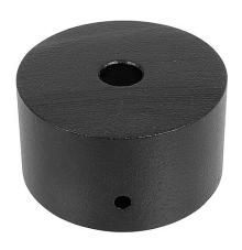
The Mega-Coupler Pipe Adapter Flush can be used to rig pipe-mounted plasma screens, projectors and speakers from overhead pipe or truss. The Mega-Coupler Pipe Adapter Flush connects onto an I-I/2" NPT threaded pipe on one end and uses a I/2" bolt to connect onto the desired mounting surface. The Mega-Coupler Pipe Adapter Flush has a I/4-20 set screw to secure the pipe threads and an inspection hole to verify that the pipe is fully inserted.
