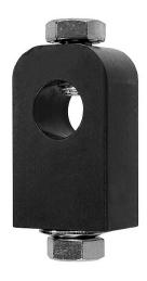
The Mega-Drop Down Slider works with The Light Source Mega-Drop Downs to locate light fixtures along the length of the Mega-Drop Down. Two 1/2"-13 × 1" long Hex Head Cap Bolts both mount the fixture and lock the fixture onto the Mega-Drop Down. A nickel plated, spring steel I inch OD Belleville spring washer is provided to act as both a tensioning and locking washer. CNC machined from aircraft grade aluminum
