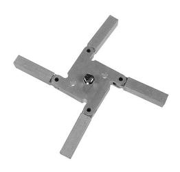
The Mega-Folding Floor Stand is a compact folding stand for placing light fixtures on the stage floor. It folds out into a stable 15" light base and folds up into a 6" square. Just fold in the appropriate legs to fit into corners, tight spots and against walls. The Mega-Folding Floor Stand has replaceable rubber feet so it won't mar the stage floor. A 1/2"-13 tpi x 1" long hex head bolt fastens the light fixture to the Mega-Folding Floor Stand. Available in either mill or black finish.
