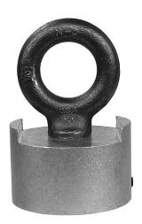
The Mega-Tie Off is used backstage for securing boom base pipes to the grid for safety. The I/2" eye bolt swivels 360 degrees. The Mega-Tie Off has I.5 NPT pipe threads and a I/2" two-way lock nut secured with permanent Loctite.
