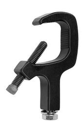
The Micro Clamp is ideal for hanging miniature fixtures like MR-16's onto a small pipe or tube. Made from high tensile aircraft aluminum. Solid design grips pipe with micro grooves, has spring loaded pan adjustment, and has 5/16" fasteners. Available in black anodized, or polished aluminum finishes.
