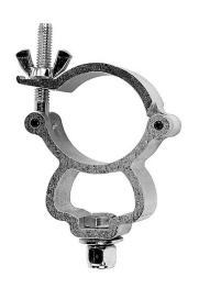
The Mini-Coupler is I" wide and fits from I.65" OD to 2" OD Tube. The Mini-Coupler uses a  $3/8'' \times 3/4$ " long Grade 5 bolt with a Belleville washer and a Nyloc nut. The Mini-Coupler has a safe working load of 330 Pounds. (I50 Kg)
