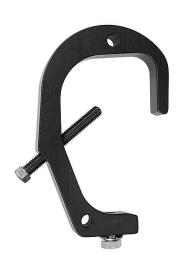
The Monstro-Clamp 4" fastens to 2-3/8" OD to 4" OD pipes. CNC cut from solid one inch thick aluminum plate. 1/2"-  $13 \times 4$ " square head bolt.
