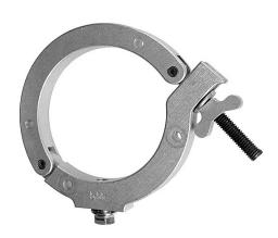
The Monstro-Couplers are designed to fit pipes larger than the standard theatrical battens. CNC machined from solid billet aircraft-grade aluminum, they are perfect for attaching to odd size pipes and tubes. Monstro-Couplers have a narrow size range of application. They are designed with a plus or minus 0.0625" tolerance on their nominal size to ensure that they will fit with the Aluminum Association pipe and tubing manufacturing tolerances. Custom sizes are available upon request.
