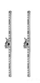
The Plasma Universal Mount supports a plasma or LCD screen on a pipe, 12", or 20.5" Truss. One Quad-Coupler 1.5 is provided to fasten per mount. The two mounting bars are bolted directly to the plasma screen with two 8mm or 10mm bolts per bar. The support bolt holes are drilled for the 50, 100, 150, 200, 300, 400, 600 mm VESA Standards. Priced per set.
