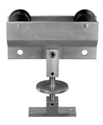
The Scenery Carrier is adjustable to fine tune the height or leveling of your flats or other scenery elements. Turnbuckle style bolt makes for quick adjustments by turning the knurled disk. Two holes are provided for #10 wood screws.
