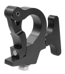
The Slim-Claw will fasten to both I-I/2" pipe (I.90" OD) and 2" OD truss tube. The Slim Claw has a 3-I/2" T-handle, so no tools are required to fasten to the pipe. Comes with  $I'' \times I/2$ "- I3 TPI Grade 5 fastener and I" diameter Belleville Spring washer.
