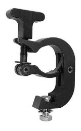
The TC Clamp will fasten from 2" OD to 1.5" OD tube. The TC Clamp has a 2-1/2" T-handle so no tools are required to fasten to the pipe.  $1.25'' \times 1/2"-13$  TPI Grade 8 fastener, Nylock Nut and 1" diameter Belleville Spring washer are provided for connecting your load. Dimensions: 4-5/8" Tx 4"W x 1-3/16" thick. Safe Vertical Working Load 450 Pounds, (200 KG). Weight is 1.22 pounds (.55 KG)
