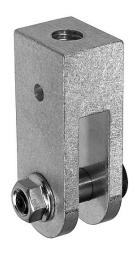
The Threaded Rod Hanger for the Mega-Batten Clamp is a I inch by 1.25 inch by 3 inch tall machined aircraft grade aluminum body with a .5 inch by .75 inch socket shoulder bolt to connect to the Mega-Batten Clamp. The design load is 1,250 pounds.
