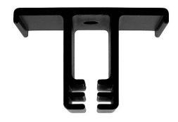
Shorter section of Mega-Track Hanger Long pre-drilled for 3/8" or 1/2" threaded rod connects M140 track to a 3/8" threaded rod while allowing for fine tuning the vertical installed height of the track.
