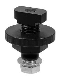
The Uni-Bolt fastens fixtures or pipes to strut channel. Insert the Uni-Bolt into the strut channel, rotate 90 degrees and spin the 2" diameter knurled disk to lock into the channel. Also available for 1.5/8" × 13/16" strut channel.
