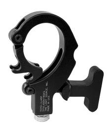
The Versi-Clamp wraps around the entire range of standard truss, from 2" OD down to 1" OD, all without marring the truss. The unique 2 position latch on the link saves time when switching from 2" truss to a small truss, just connect to the second latch for the smaller sizes. The quick release handle takes only 2 turns to be able to drop the locking mechanism, and release the clamp from the truss.
