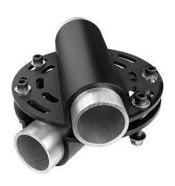
The new Mega-Gridlock Diagonal XL provides a solution for pipes that need to cross at varying angles. Multiple curved slots allow for precise positioning from 0° to 90°. The Mega-Gridlock Diagonal XL works with 2 bolts or 4 bolts, depending upon the configuration of the pipes. With 4 bolts installed, the WLL is 800 lbs. The Mega-Gridlock Diagonal XL is a great option for versatility as well as accuracy in pipe installations.
