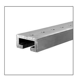
The XYZ Channel and the XYZ Mount make installing LED video walls a breeze. The 606 IT6 aluminum alloy channel is pre-drilled on one inch centers for number I2 flathead screws to allow easy mounting to I6" and 24" on center studs. The XYZ mount slides in from the side to any desired location and is locked in place with a set screw. Available in two lengths, I800 mm and 2400 mm, to match most LED panels.
